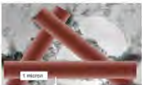
Fig. 3: Red-D Ultra has been specifically engineered to have an average pore size of 2 microns and a mean flow pore of 0.7 microns. This allows the charge field created by the alumina fibers to effect the total volume of the individual pores as well as virtually the entire void volume of the
